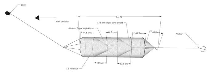
Figure 10. Schematic of commercial hoop net
