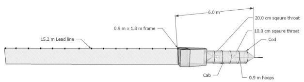
Figure 13. Schematic of modified fyke net
