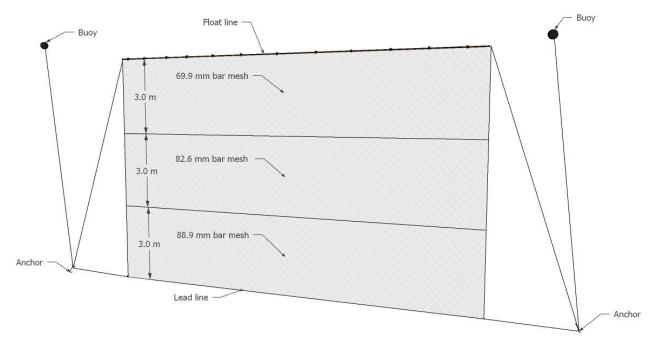
Figure 7. Generalized schematic of a deep-water gill net.
