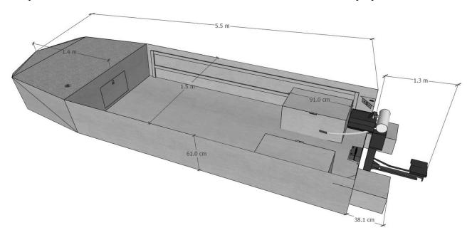
**Figure 19.** *Schematic of the shallow drive boat.*
