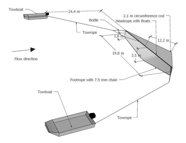
Figure 6. Generalized schematic of a trawl.
