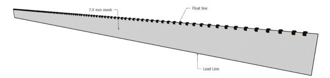
**Figure 17.** *Generalized schematic of a block net.*
