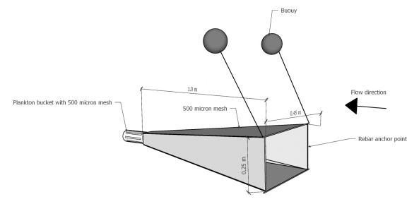
**Figure 15.** *Generalized schematic of a drift net.*
