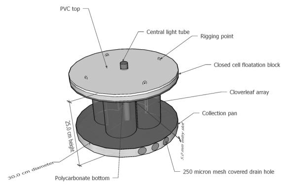
Figure 16. Schematic of Quadrafoil light trap
