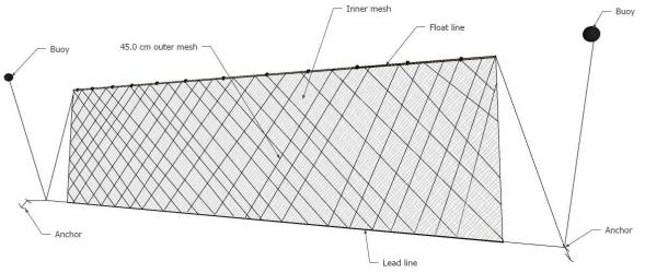
**Figure 9.** Generalized schematic of a commercial trammel net.
