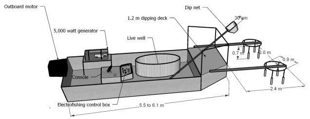
**Figure 1.** *Schematic of electrofishing boat.*
