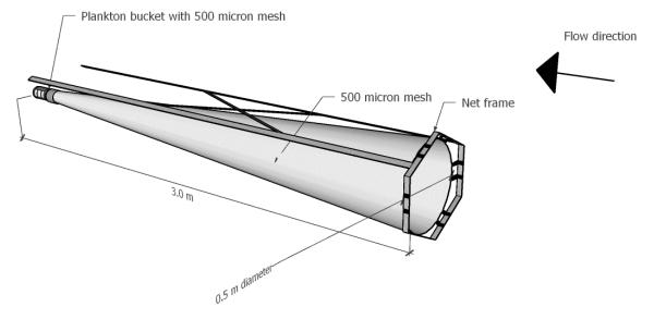
**Figure 14.** *Generalized schematic of a pushnet.*
