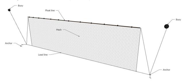
**Figure 8.** Generalized schematic of a commercial shallow gill net.
