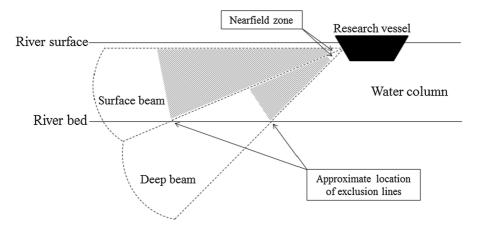
**Fig. 2** Schematic (not to scale) depicting the orientation of the two hydroacoustic beams in the water column. Both transducers were deployed 0.4 m below the river surface. Maximum beam length was 50 m but exclusion lines were drawn at the point where the beams intersect the river bed. The areas in which
