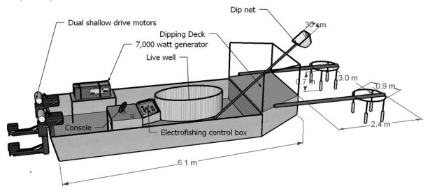
**Figure 2.** *Schematic of the shallow drive electrofishing boat.*
