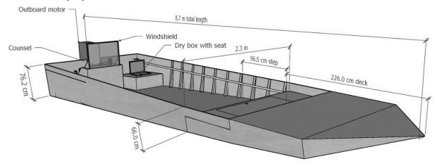
Figure 18. Generalized schematic of netting boat.
