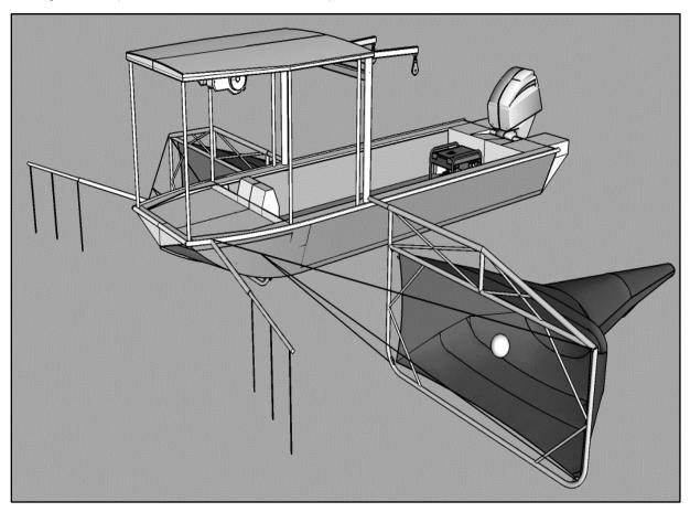
Figure 4. Schematic of electrified Paupier trawl
