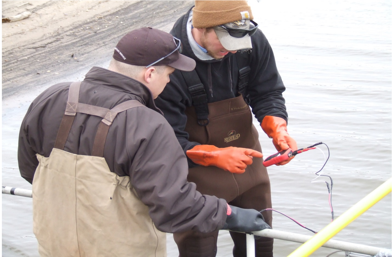
Image 1: Skyler Schlick of Columbia FWCO works with Kjetil Henderson of Wilmington USFWS to map the electrical field created by an electro-fishing boat.
