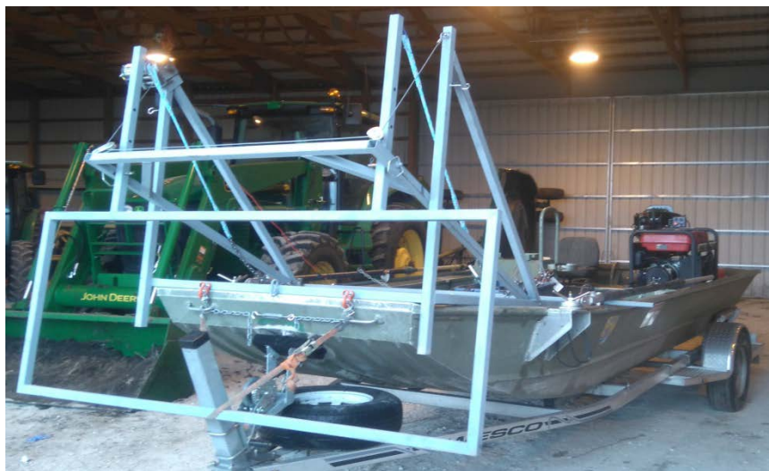
Image 1: Skyler Schlick of Columbia FWCO works with Kjetil Henderson of Wilmington USFWS to map the electrical field created by an electro-fishing boat.
