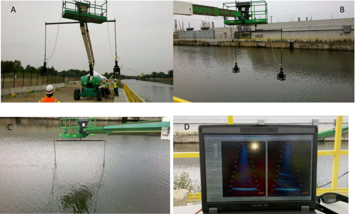
Figure 4. Two DIDSON units being deployed into the CSSC using a telescopic boom lift (A-C) and the two DIDSON units being operated on one computer (D).
