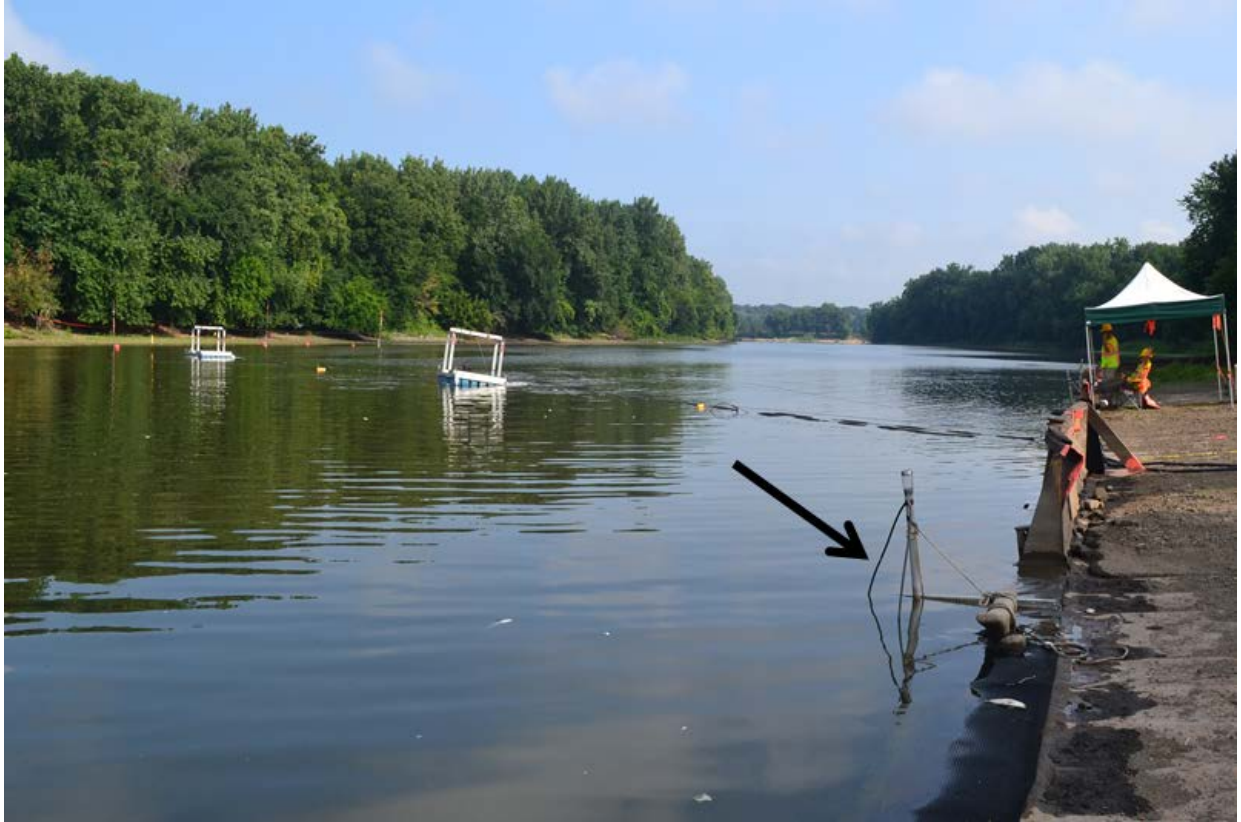
Figure 13. Image of the first test site for water gun barrier observations in the channel connecting Hanson Materials Sand and Gravel Mine to the Illinois River. Water guns are suspended from pontoons floating mid-channel. A hydroacoustic transducer mount can be seen in the lower left corner (black arrow).
