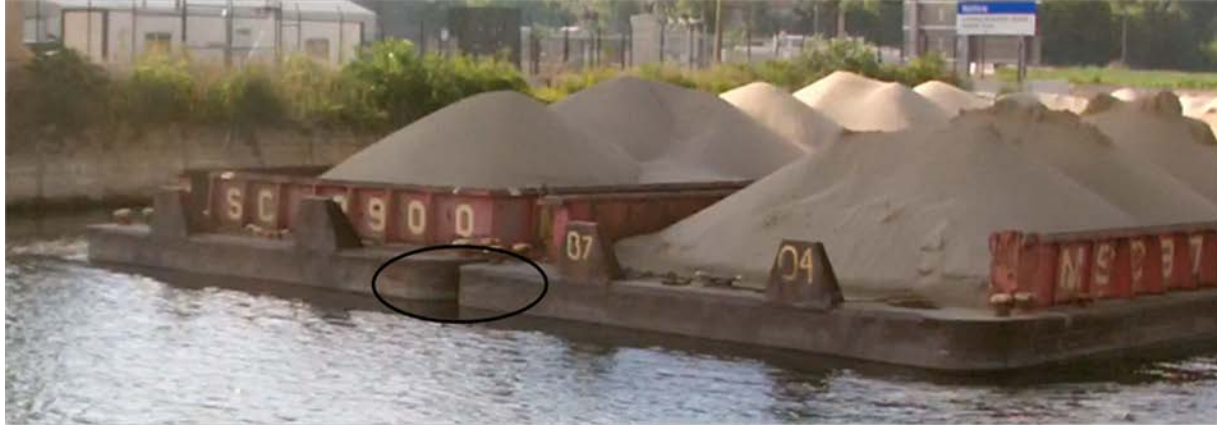
Figure 4. Picture of the front of a rake-to-rake barge configuration traversing the Electric Dispersal Barrier with the square ends in the front. The circle denotes the small void space that two live fish swam into and remained inside beyond the barrier.
